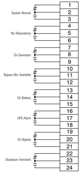
Figure 5-11. Supervisory Contact Module II TB2
